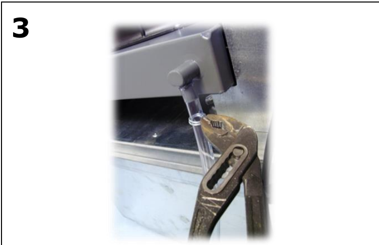
Pinch the collar to open it and slide it along the pipe
